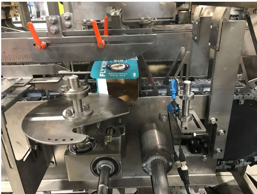
Figure 22 - Flap Sequence #1 – Major Flaps Being Controlled, (Stock Photo)
