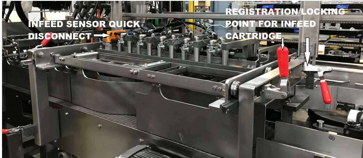
C110 - #5A - Infeed Lane Cartridge mounted In Position
