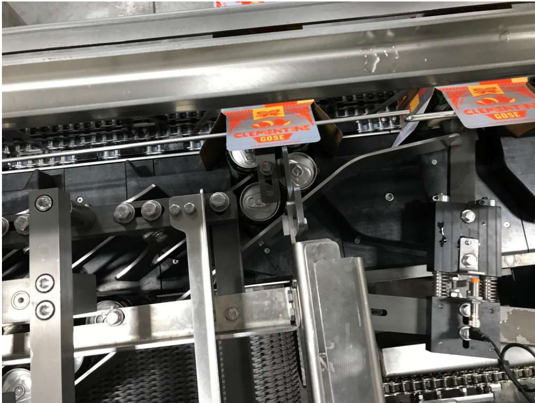
Figure 51 - Load Sequence #12 –Pattern Getting Plowed Into Carton, (Stock Photo)
