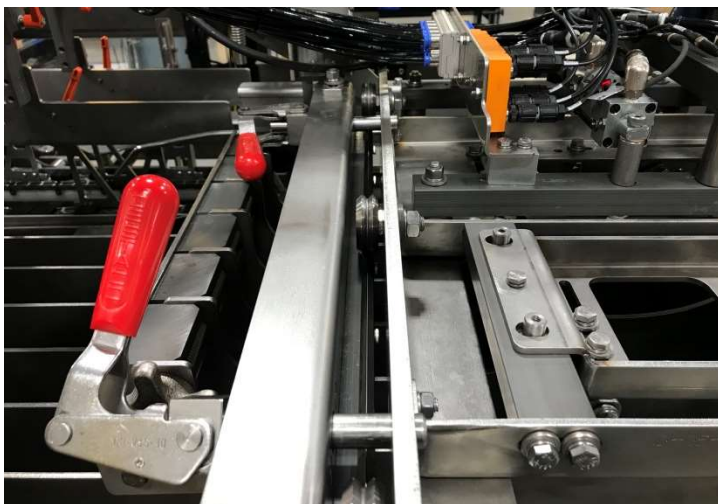
C117 - #5H - Infeed Lane Cartridge Upstream Locking Mechanism Disengaged
