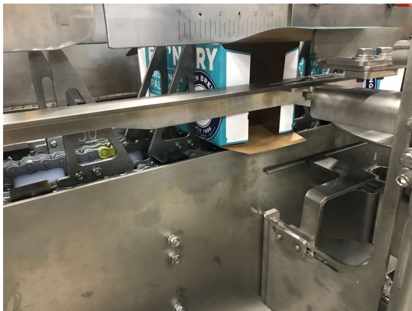
Figure 28 - Flap Sequence #7 –Non Load Side Upstream Minor Getting Tucked Closed, (Stock Photo)
