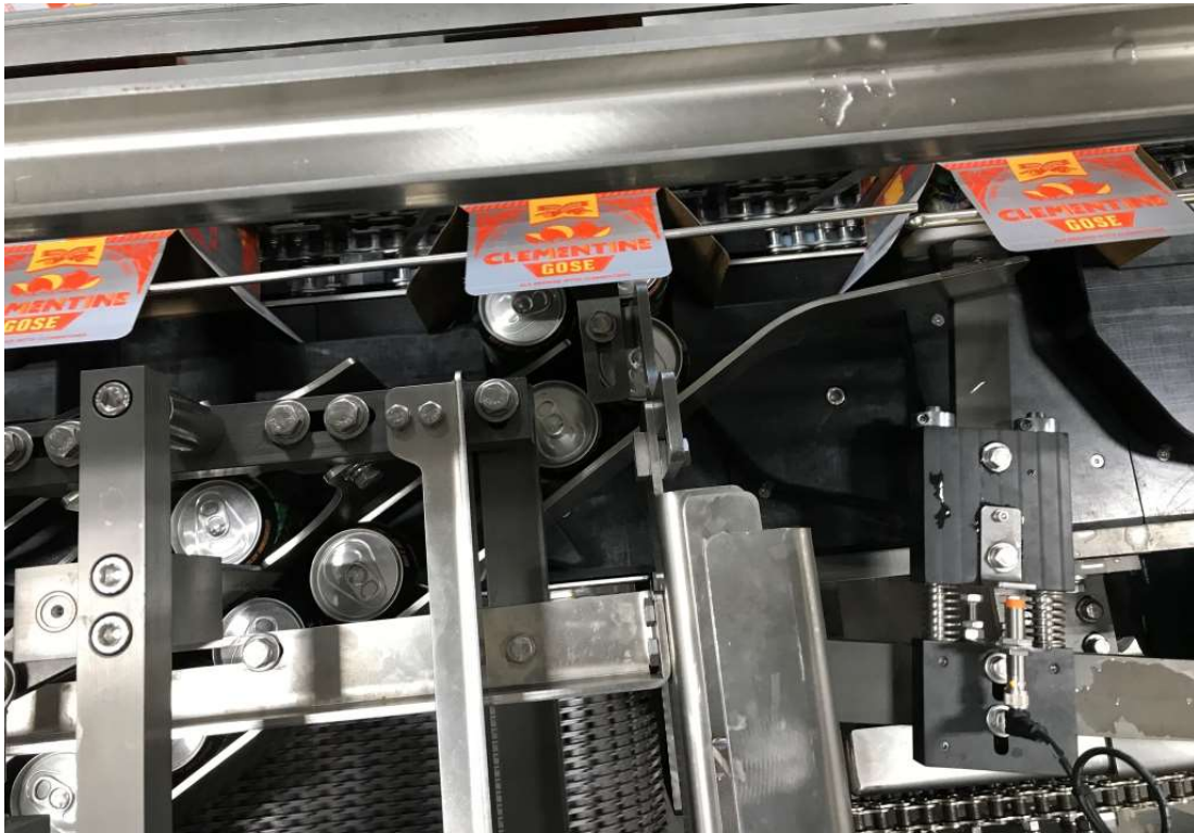
Figure 45 - Load Sequence #6 –Pattern In Bucket, Moving Into Carton
