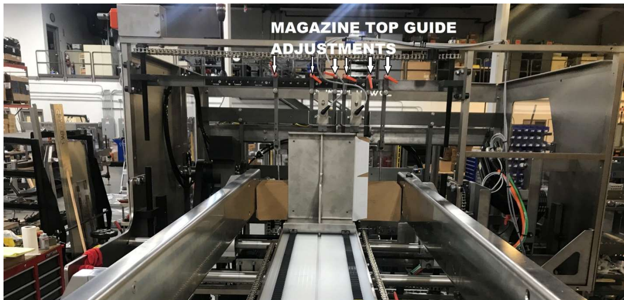
Figure 129 - C #7 – Magazine Top Guide Clips
