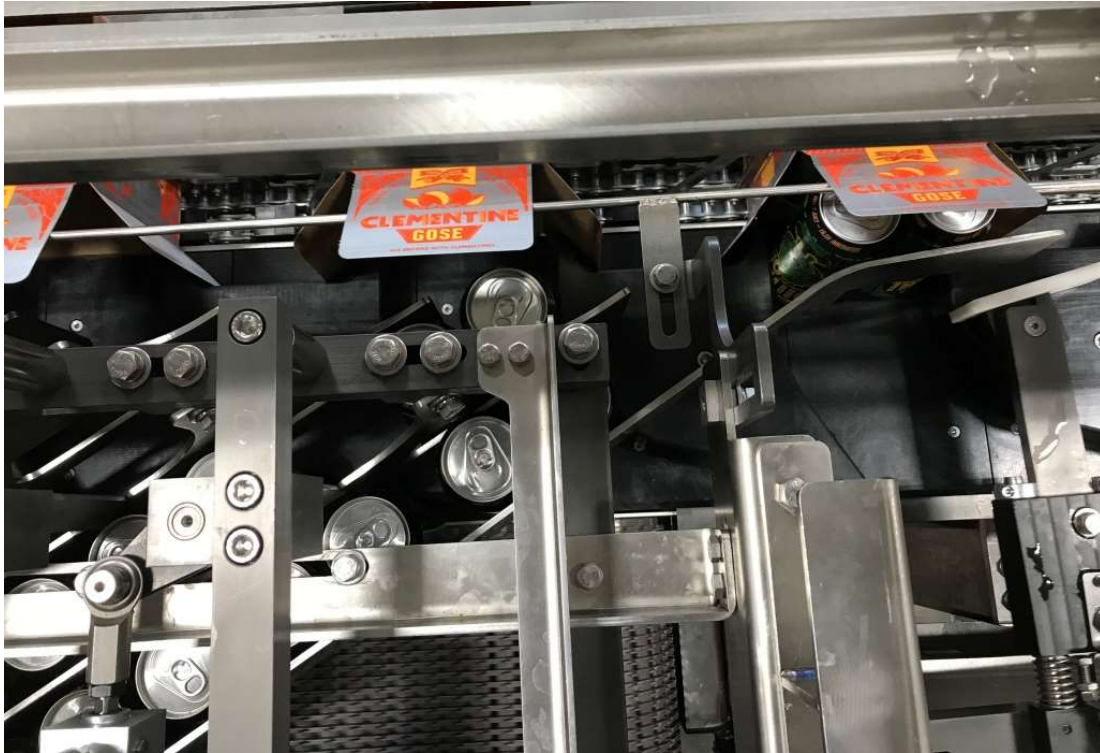
Figure 43 - Load Sequence #4 –Pattern Proceeding Into Bucket
