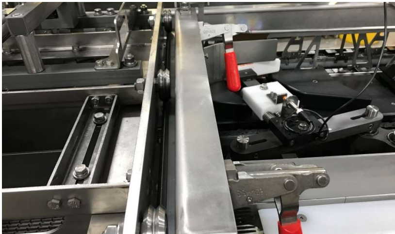
C119 - #5J - Infeed Lane Cartridge Downstream Locking Mechanism Disengaged
