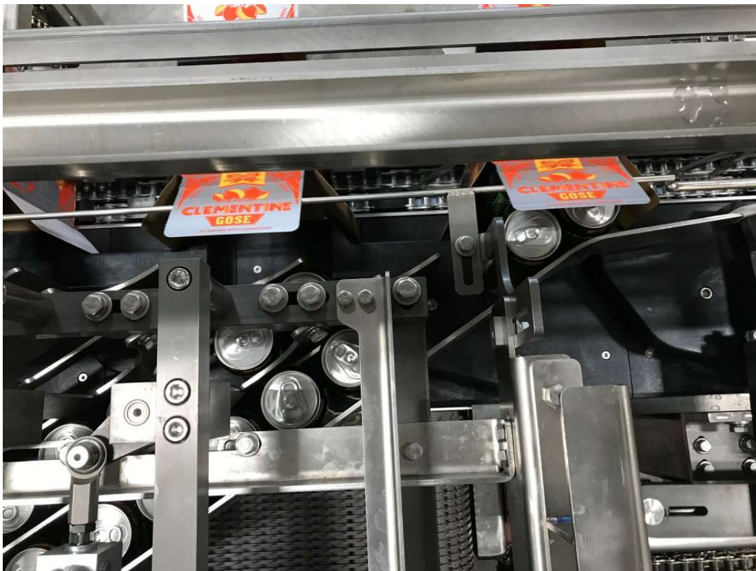
Figure 42 - Load Sequence #3 –Pattern Proceeding Into Bucket
