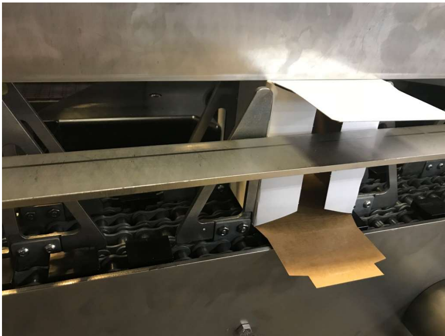
Figure 32 - Flap Sequence #11 – Wedge Moved Up To Load Side Upstream Minor Flap, (Opposite Hand)
