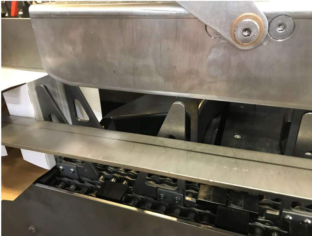
Figure 29 - Flap Sequence #8 – Wedge Moving By Load Side Downstream Minor Flap, (Opposite Hand)
