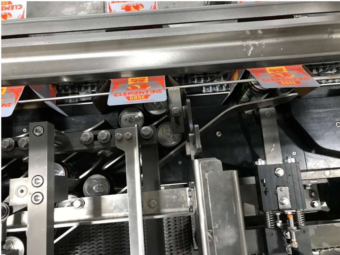
Figure 44 - Load Sequence #5 –Pattern In Bucket, Next Pattern Collating
