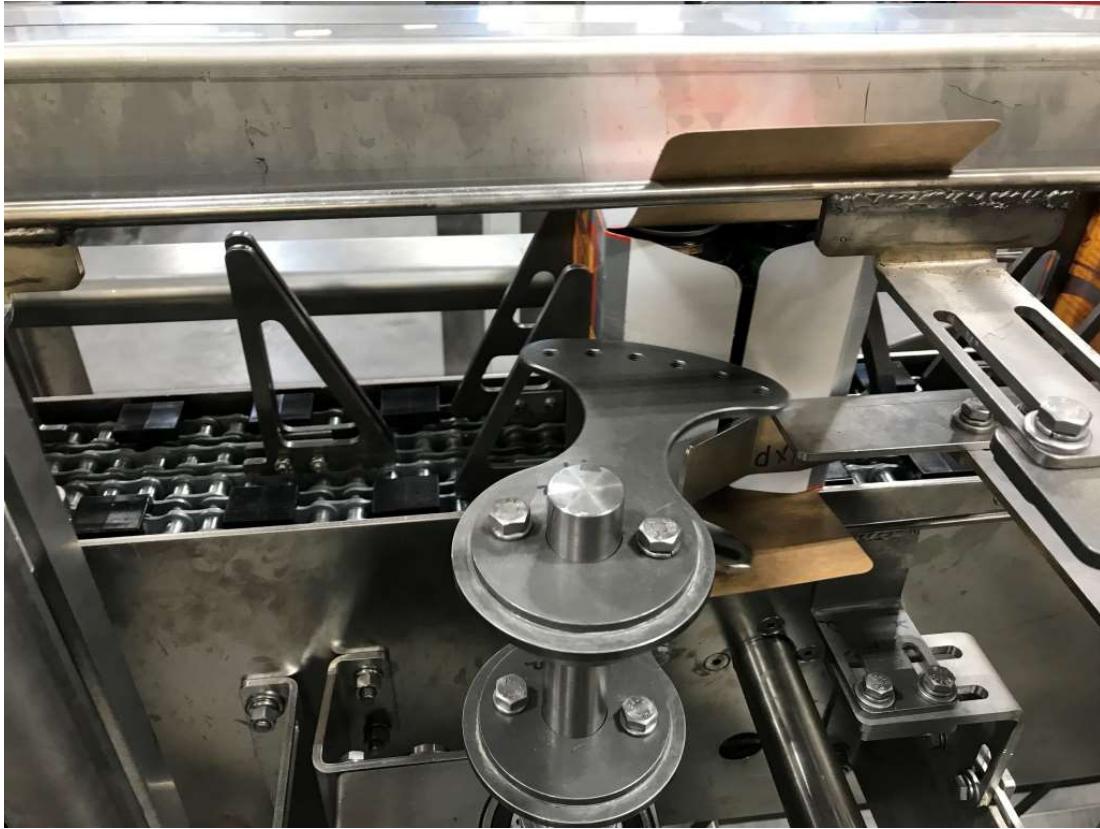
Figure 57 - Forming Sequence #3 – Leading Minor Flaps Plowed Trailing Minors Getting Tucked
