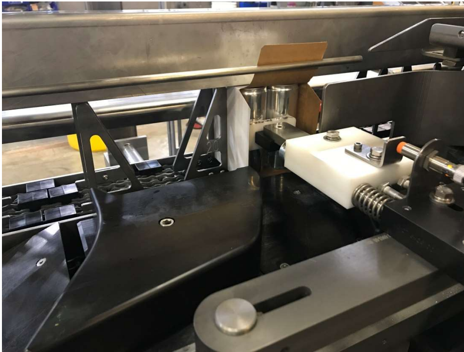
Figure 53 - Load Sequence #14 –Can Pusher Extended, (Opposite Hand)
