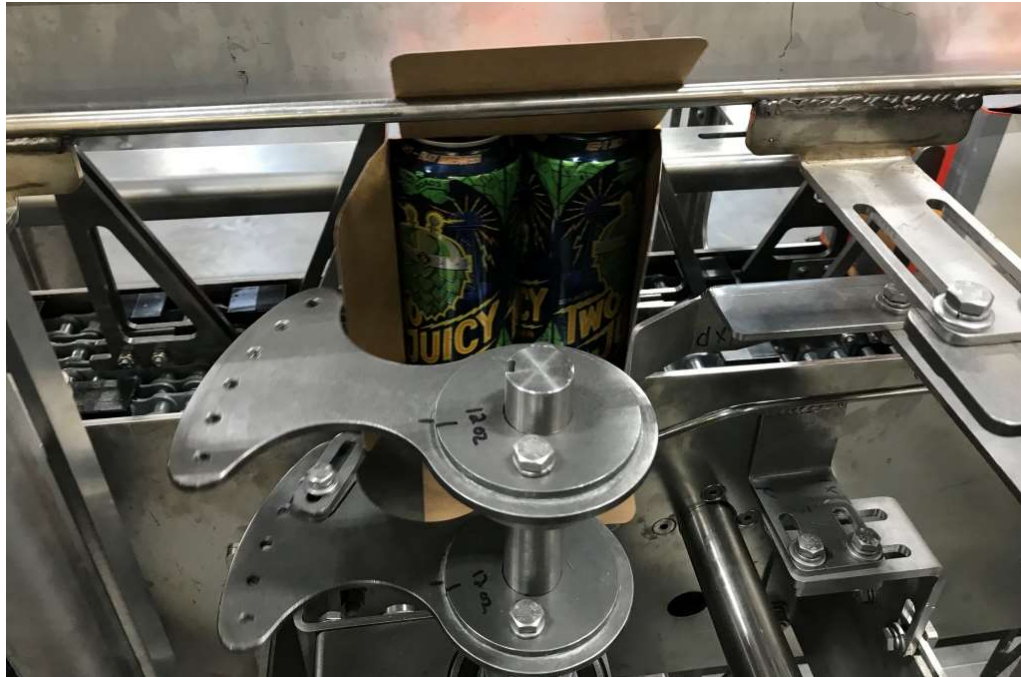
Figure 55 - Forming Sequence #1 – Leading Minor Flaps Being Plowed
