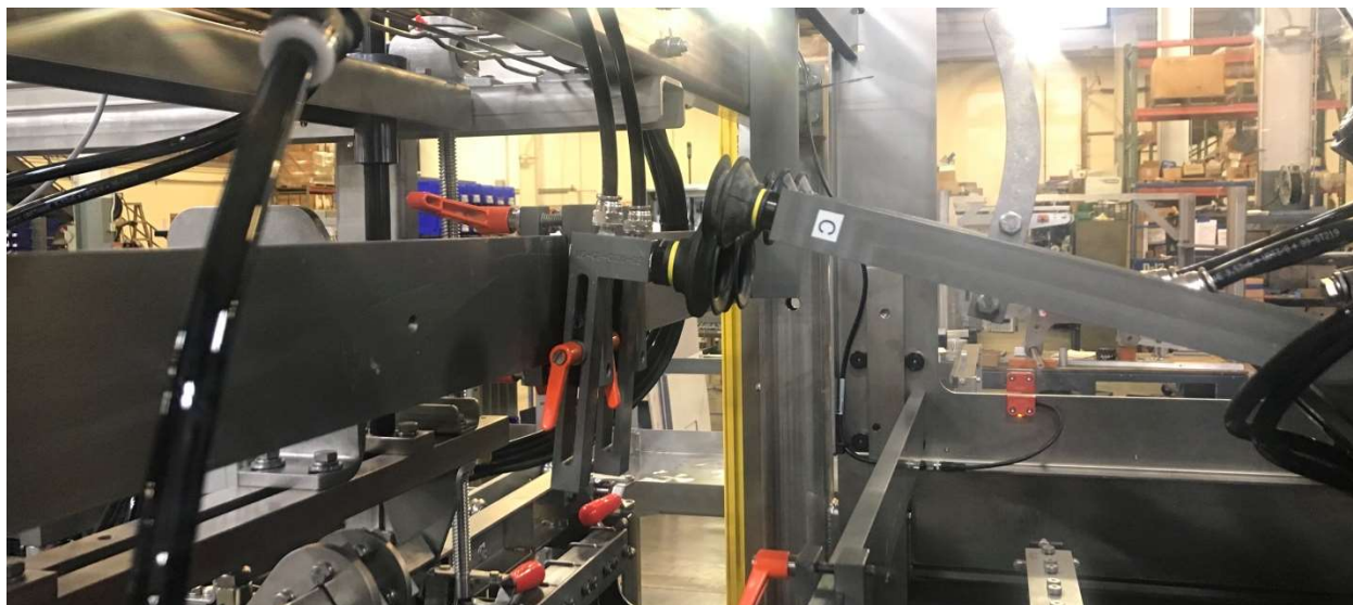
Figure 6 - Vacuum Pre Break Position
