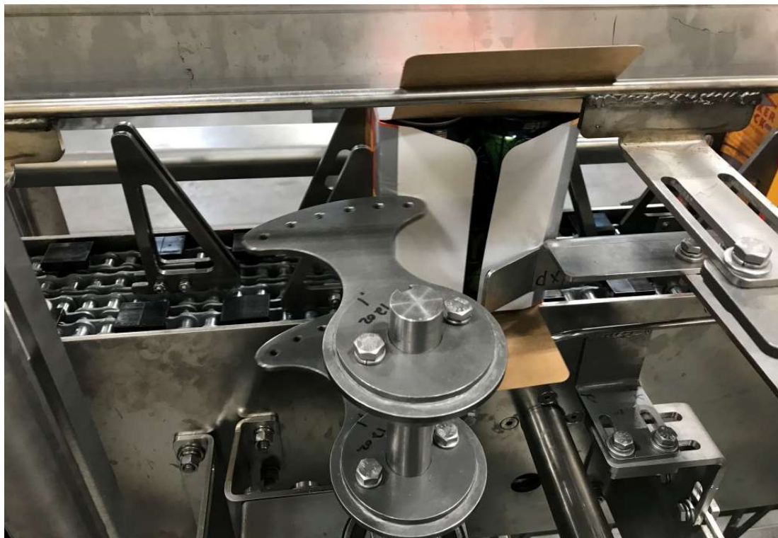
Figure 56 - Forming Sequence #2 – Leading Minor Flaps Being Plowed
