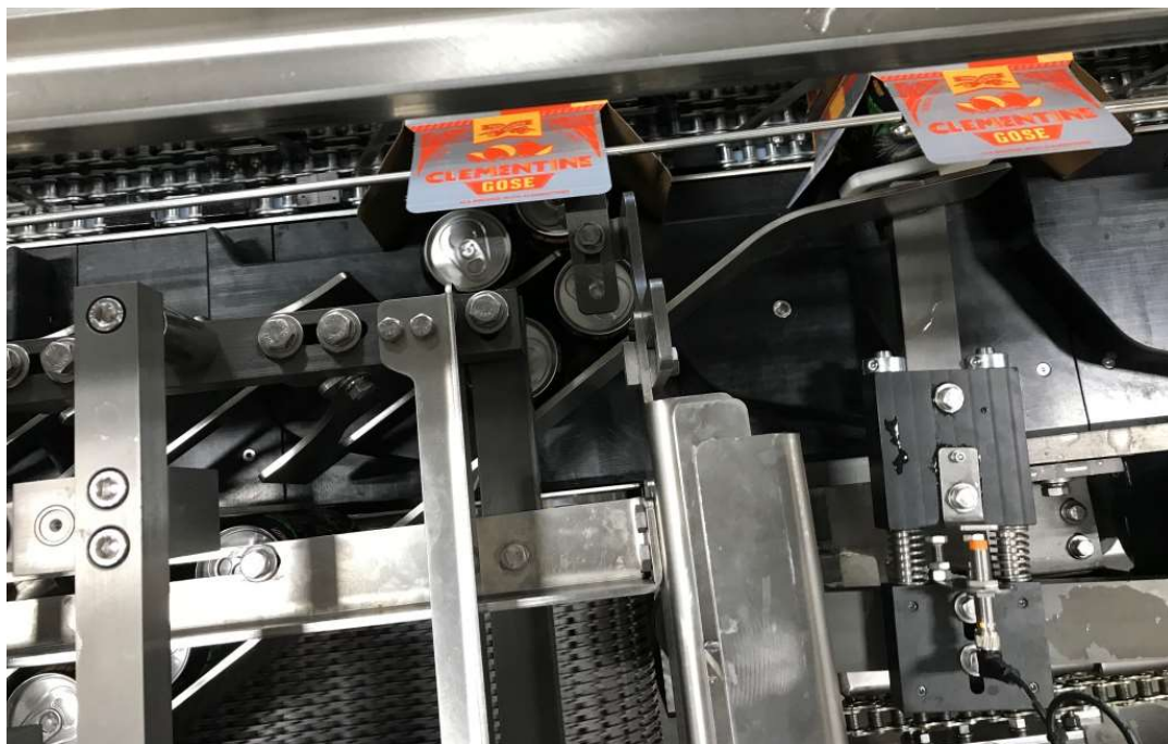
Figure 50 - Load Sequence #11 –Pattern Getting Plowed Into Carton, (Stock Photo)
