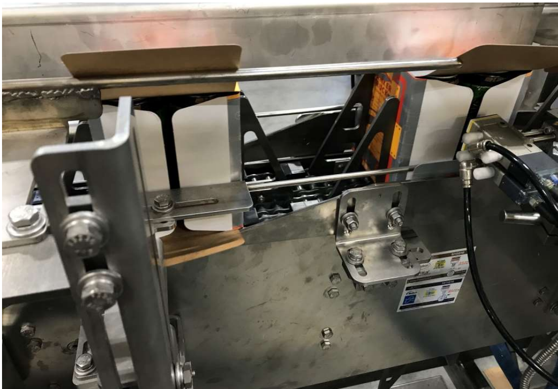
Figure 58 - Forming Sequence #4 – Minor Flaps Plowed/Tucked In
