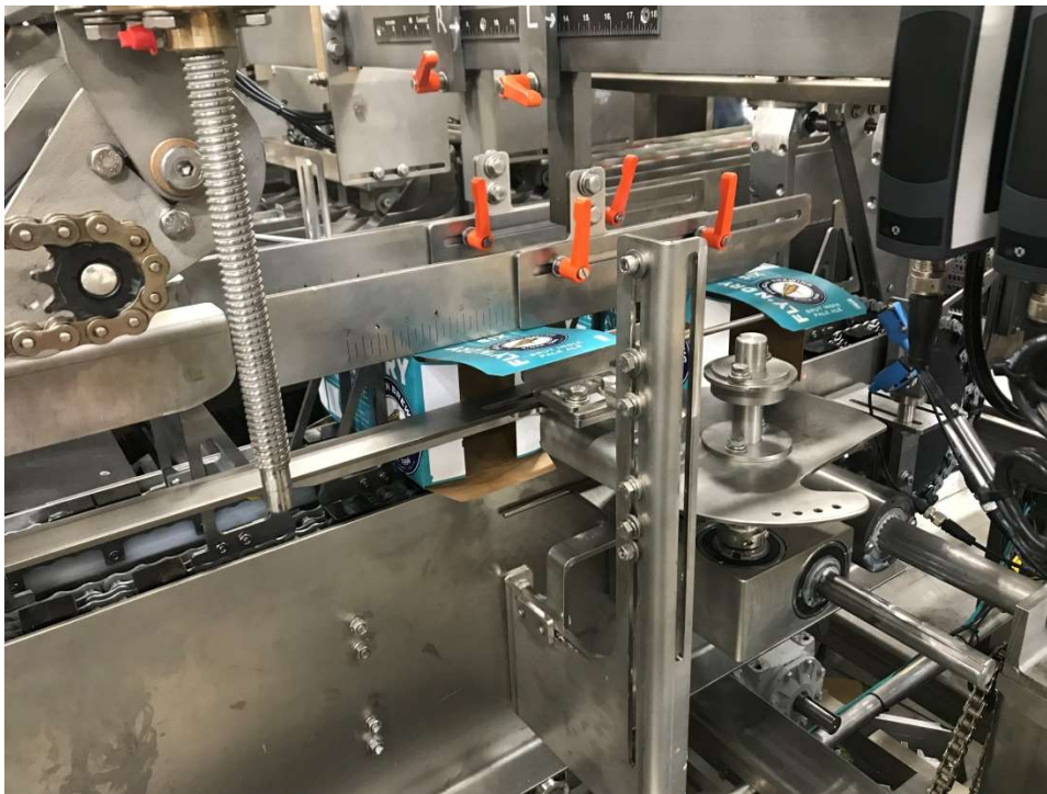
Figure 26 - Flap Sequence #5 –Non Load Side Upstream Minor Getting Plowed Closed, (Stock Photo)
