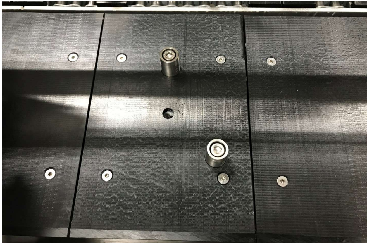
125 - #6B – Change Out Wedges – Wedge Locating Plate,
