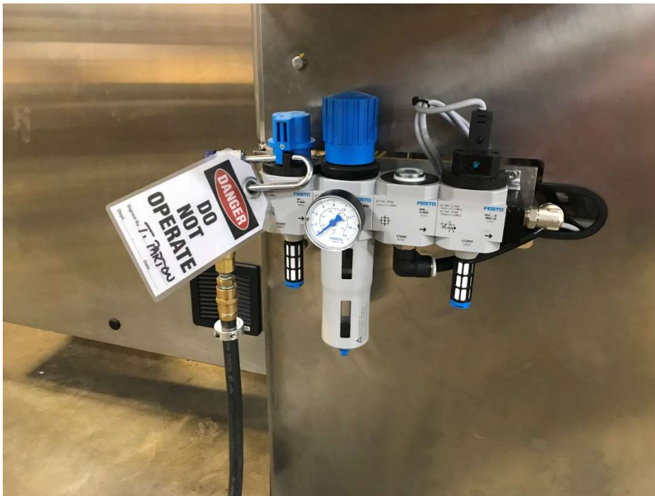
Figure 202 - Pneumatic Lockout/Tag Out
