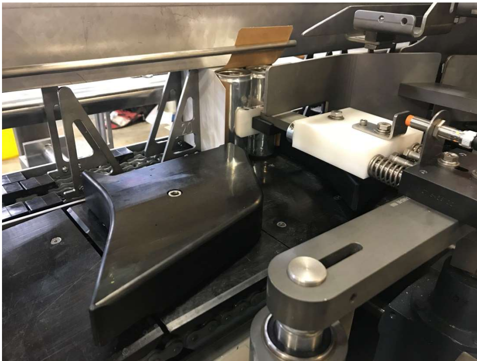
Figure 52 - Load Sequence #13 –Pattern Getting Pushed Into Carton, (Opposite Hand)
