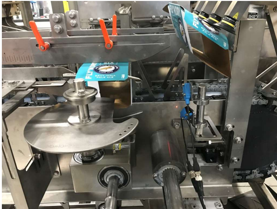
Figure 23 - Flap Sequence #2 – Leading Minor Flap Being Plowed, (Stock Photo)
