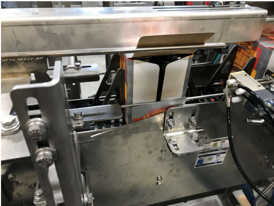
Figure 60 - Forming Sequence 6 –Bottom Majors Being Plowed Up
