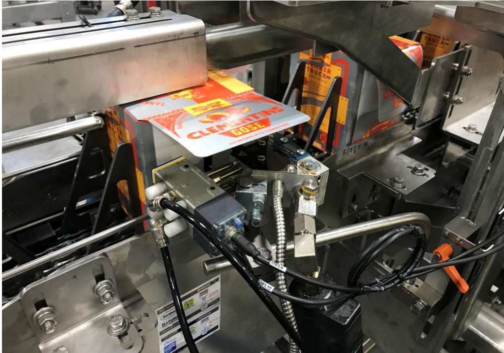
Figure 61 - Glue and Compression Sequence 1 - Carton Glue Starting
