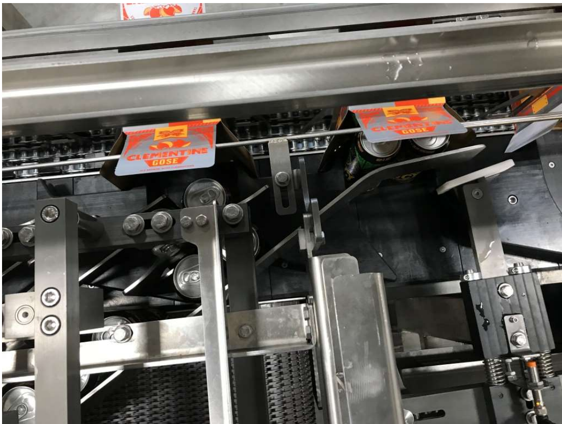
Figure 48 - Load Sequence #9 –Pattern Moving Into Carton
