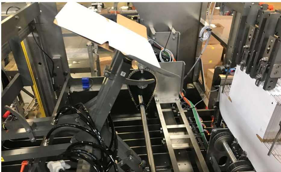
Figure 10 - Carton Erect Sequence #3
