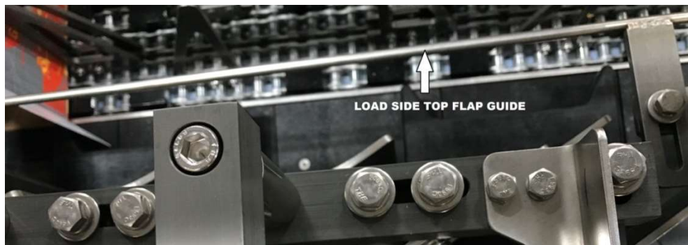
Figure 142 - C #18 – Front Top Guide Plow
