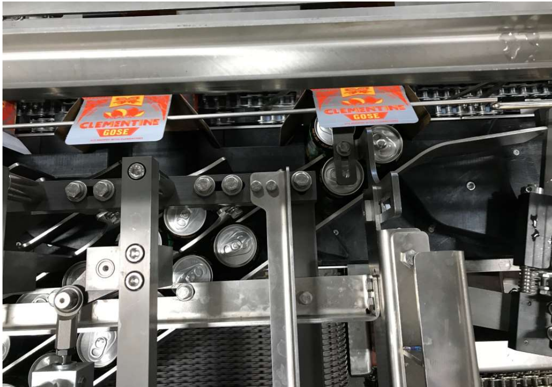
Figure 41 - Load Sequence #2 –Lane 1 Gate Open
