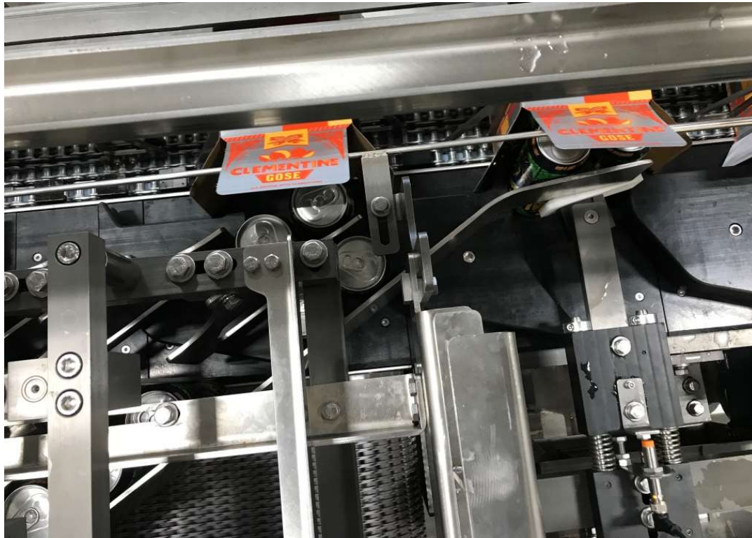
Figure 49 - Load Sequence #10 –Pattern Moving Into Carton, (Stock Photo)
