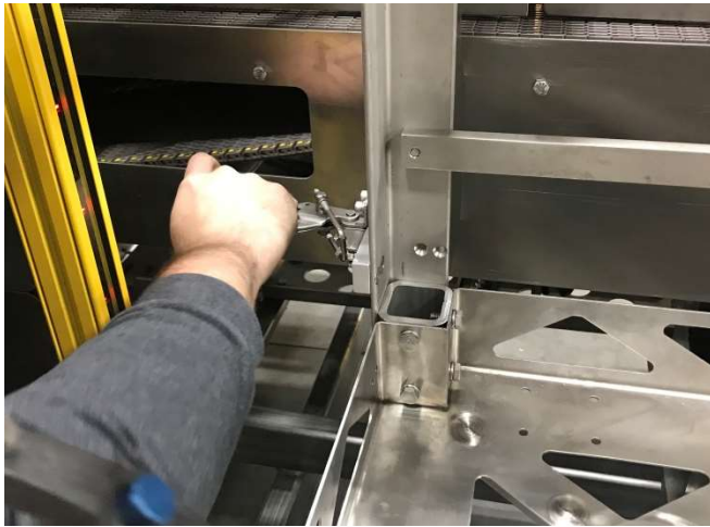
C121 - #5L - Cartridge Cart Locking Points Upstream Side,
