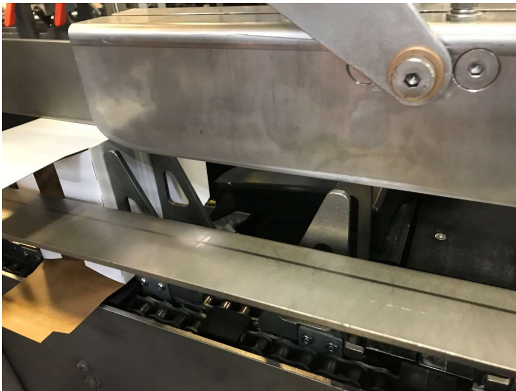
Figure 30 - Flap Sequence #9 – Wedge Moved By Load Side Downstream Minor Flap, (Opposite Hand)
