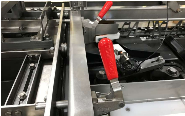
C118 - #5I - Infeed Lane Cartridge Downstream Locking Mechanism Engaged
