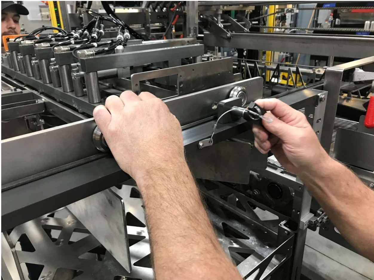
C122 - #5M - Infeed Lane Cartridge On Cart, Locking Pin Being Inserted
