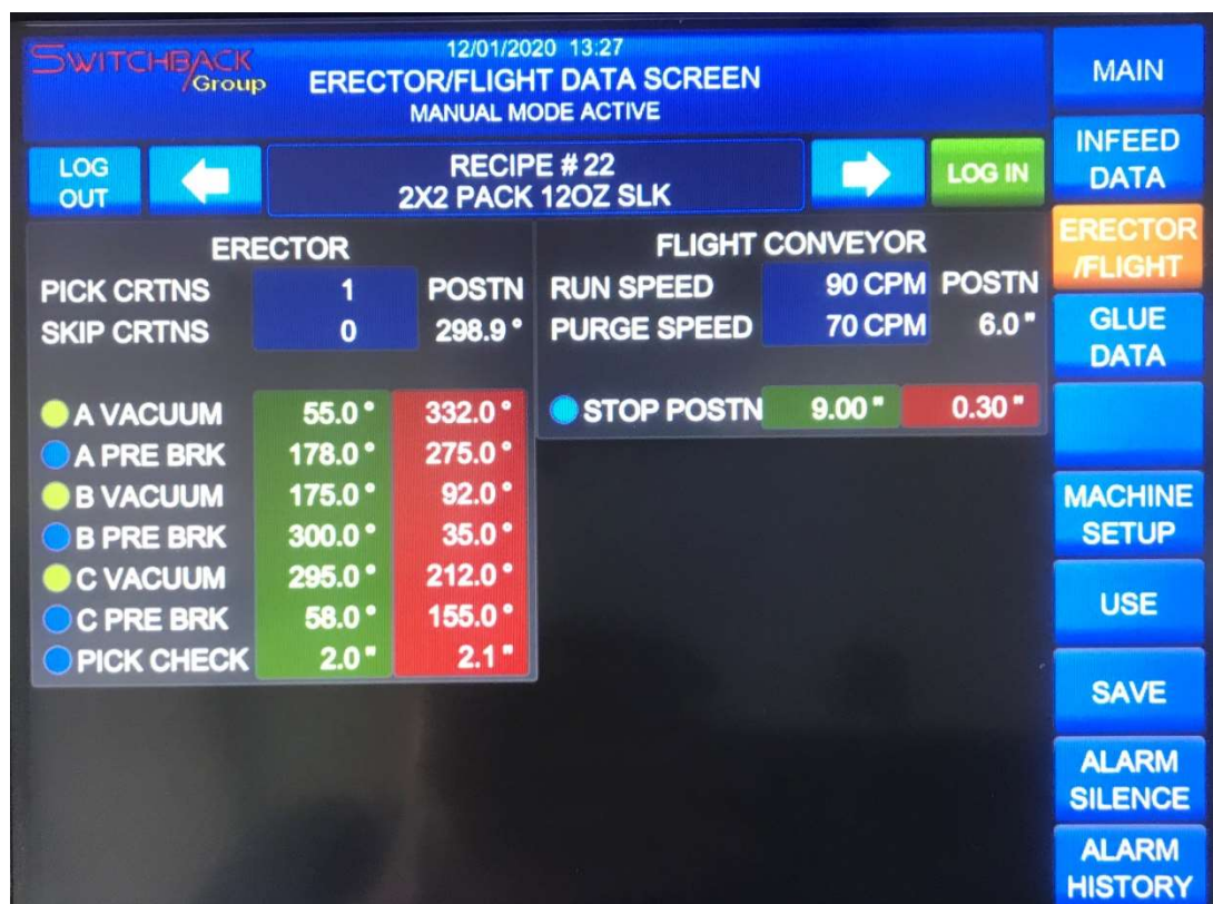
Figure 186 – Original Settings Recipe #22 Erector/Flight Data
