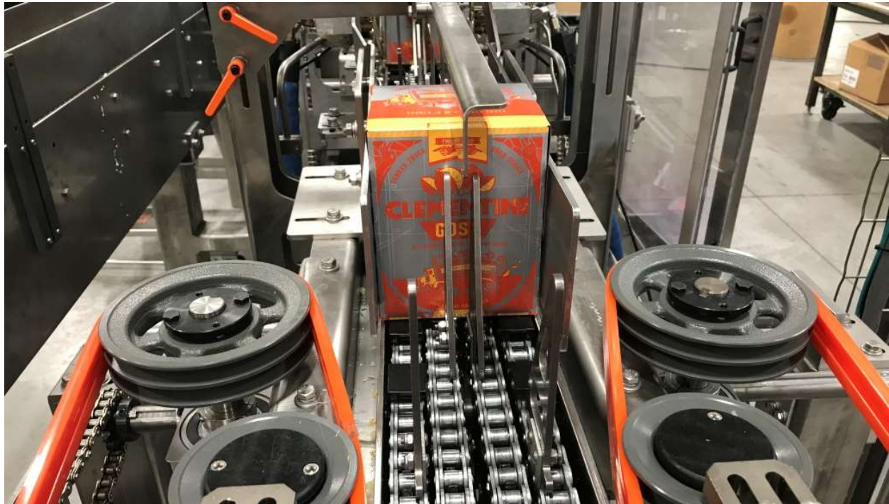
Figure 67 - G&C Sequence 7 – Carton in Compression, End View
