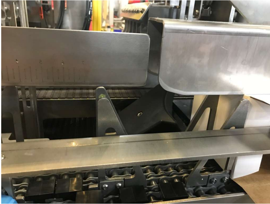
Figure 31 - Flap Sequence #10 – Wedge Moving Up To Load Side Upstream Minor Flap, (Opposite Hand)
