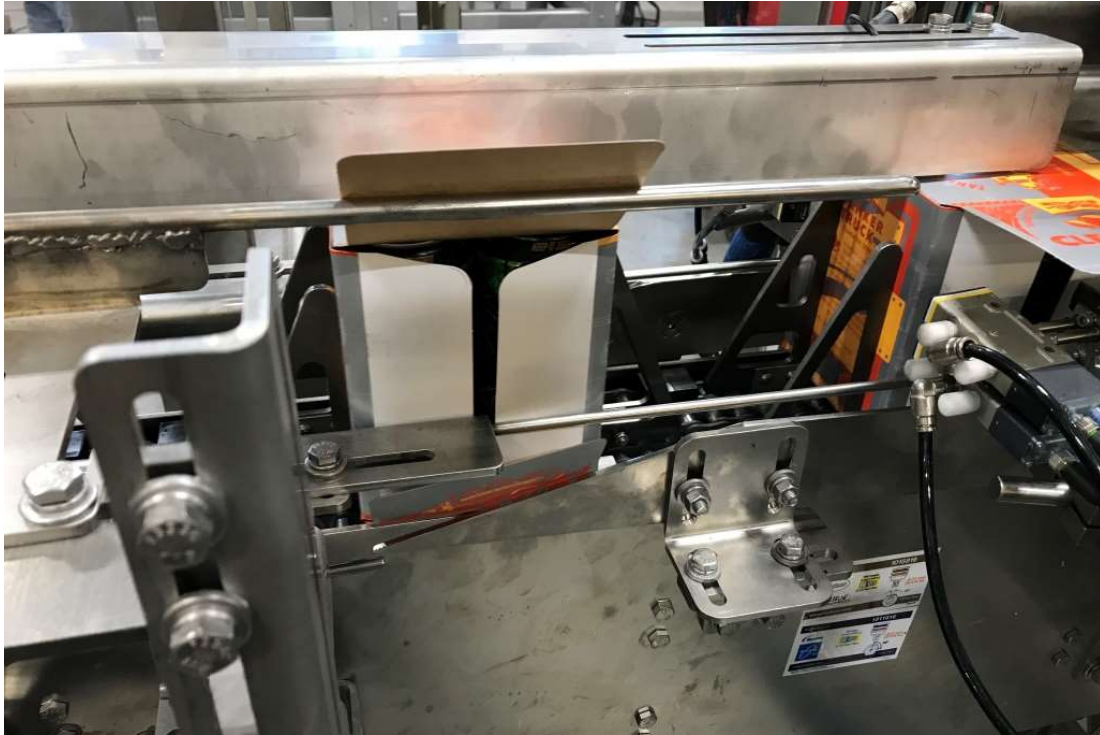
Figure 59 - Forming Sequence #5 –Bottom Majors Being Plowed Up
