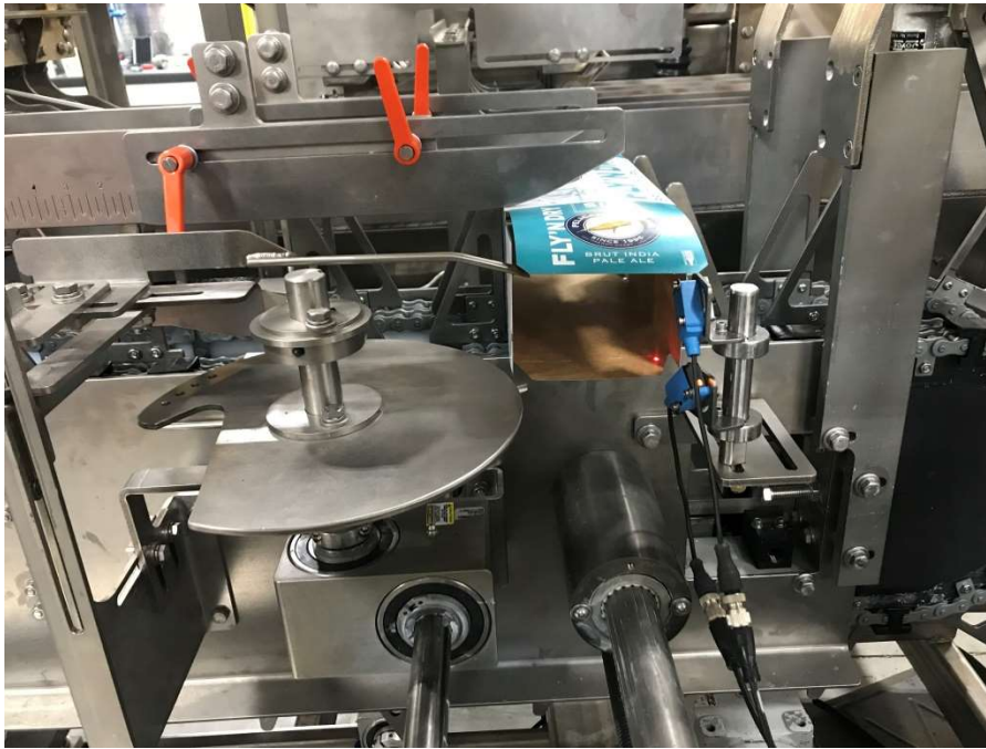
Figure 21 - Carton Erected, (Stock Photo)
