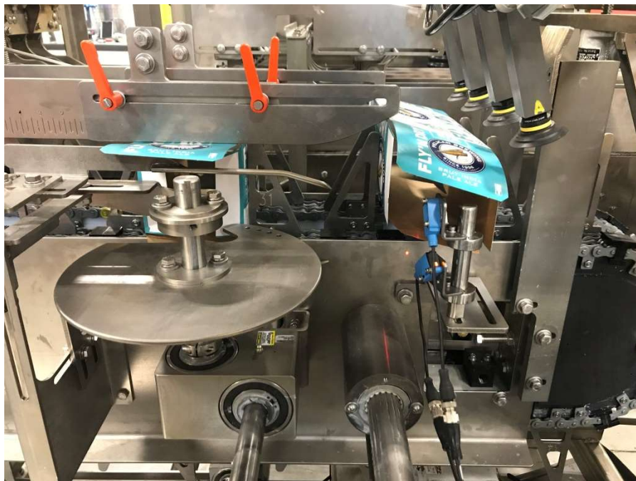
Figure 24 - Flap Sequence #3 – Leading Minor Flap Being Plowed Further, (Stock Photo)
