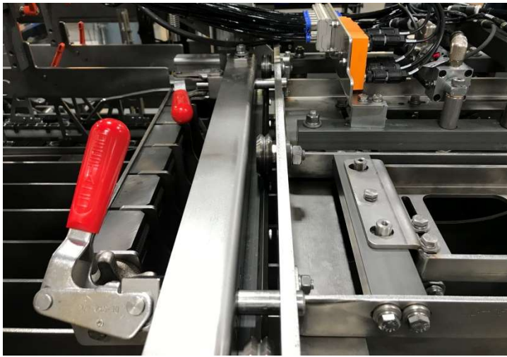
C116 - #5G - Infeed Lane Cartridge Upstream Locking Mechanism Engaged
