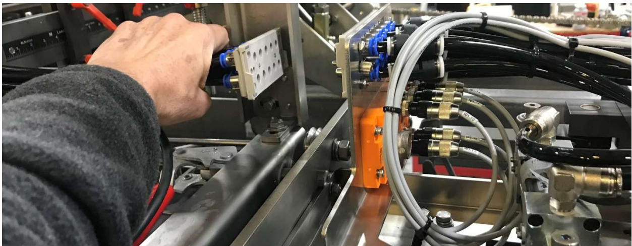
C114 - #5E - Infeed Lane Cartridge Pneumatic Quick Disconnect Being Removed
